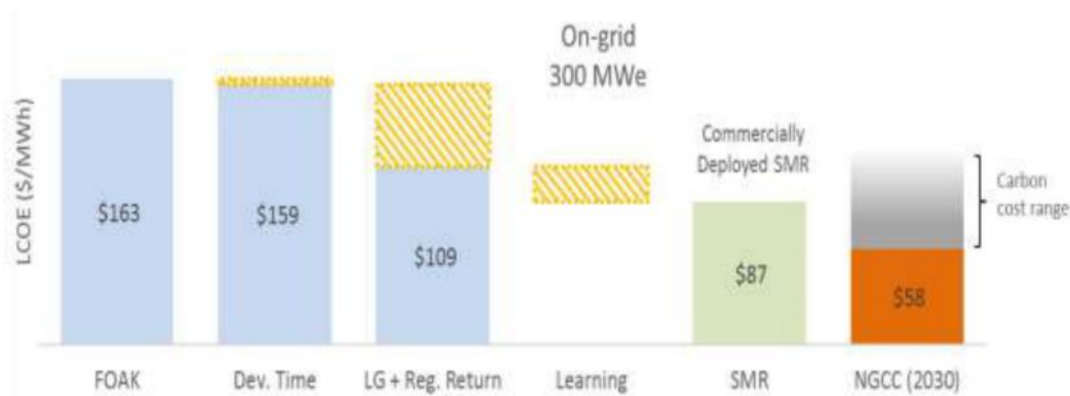
Figure 15 Estimated cost reductions from first SMR to commercial deployment (Source: SMR Roadmap)
